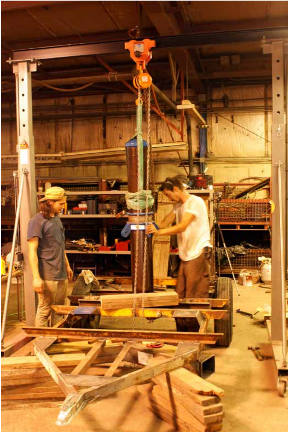
The Fairmont was painstakingly refurbished and brought back to working order, although it was modified for paved roads rather than railroads. The modifications entailed the addition tires and outriggers for stability.
